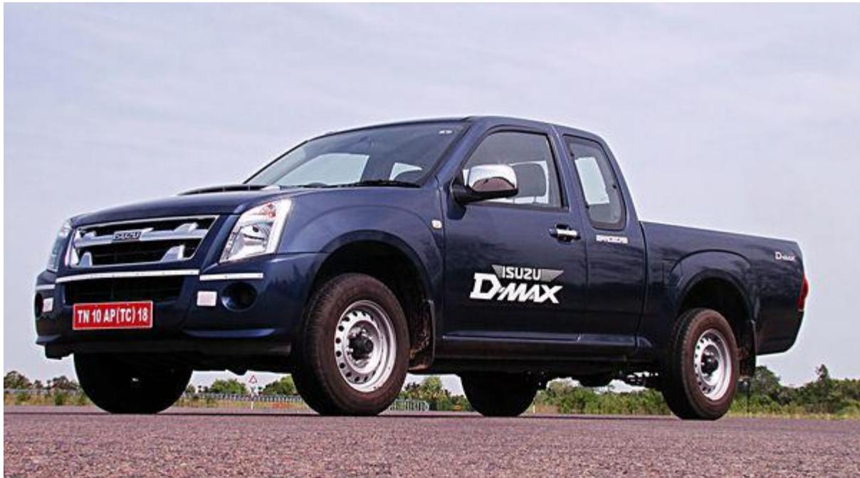
It has a straight cut design. Gets chrome finish on the toothed radiator grille. It has body coloured bumpers and provisions for fog lamp housing. Short hood also features an air intake scoop. Side mirrors have chrome too. These mirrors cannot be adjusted from inside but externally. An internal adjustment setting is in the pipeline and will feature soon.
