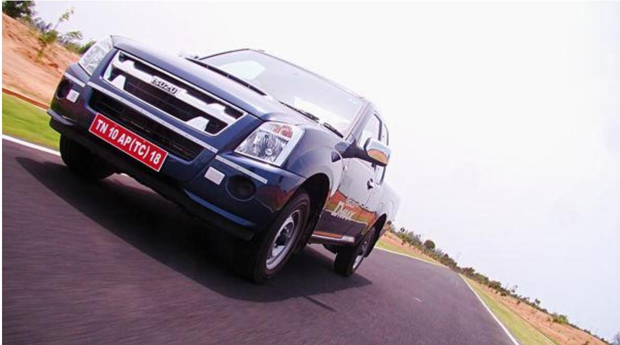
Dimensionally, it is smaller than the Mahindra Scorpio Getaway and Tata Xenon XT. The cabin feels placed at a lower height than the other two. This given an advantage as the resistance to oppose air flow is lesser. Even at speeds above 140kmph, it felt extremely stable and confident. It gets disc brakes on the front and drum on the rear. The company officially offers an option of Dunlop and Bridgestone tyres.
